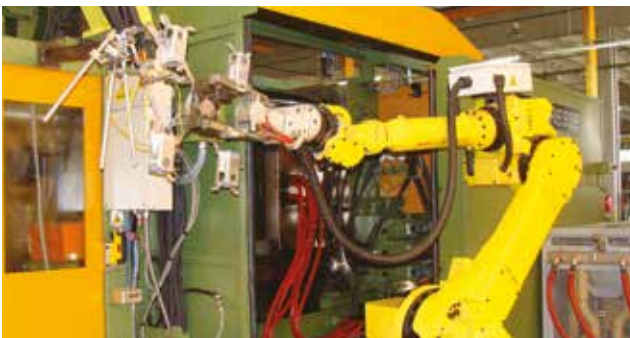
Parts being extracted by robot
