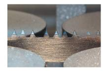
Most of the blades are produced in hardpoint finish and are rust protected
